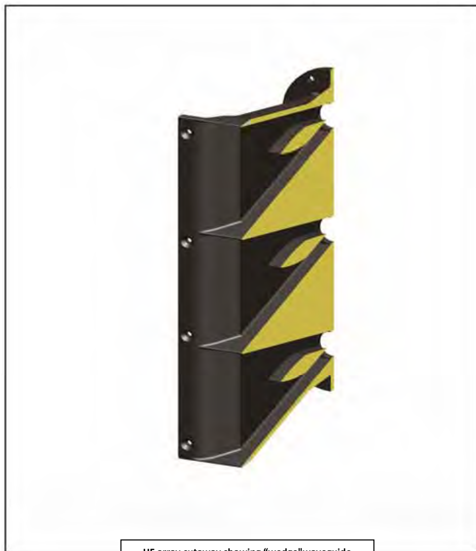
HF array cutaway showing "wedge" waveguide
