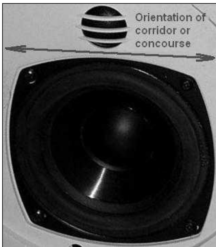
2-way ceiling loudspeaker orientation
